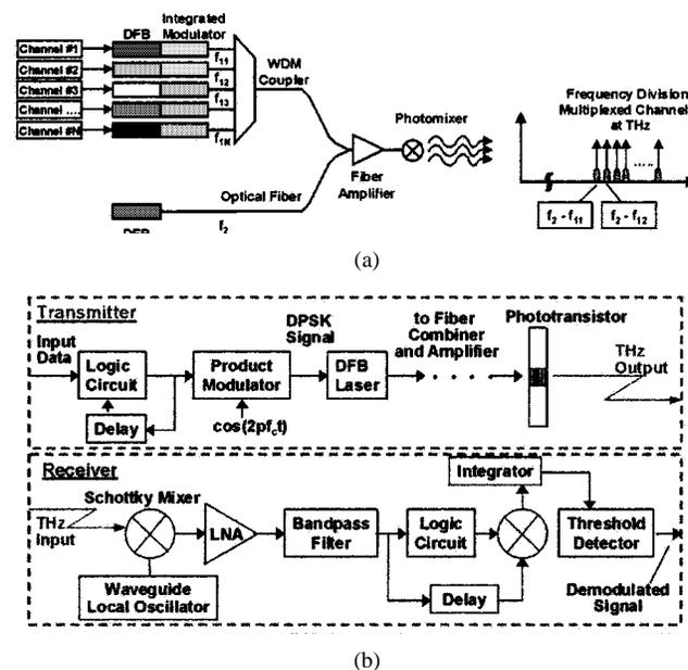
Fig. 10. (a) Optically diphed terahertz transmitter source based on 1.5- $\mu\text{m}$  fiber technology and terahertz power generation through photomixing. (b) Gigabit data-rate transmit/receive module based on this technology (courtesy of [52]).
