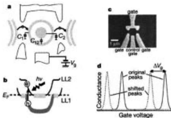
Fig. 17. Komiya quantum-dot single-photon detector concept (courtesy of [137]).
