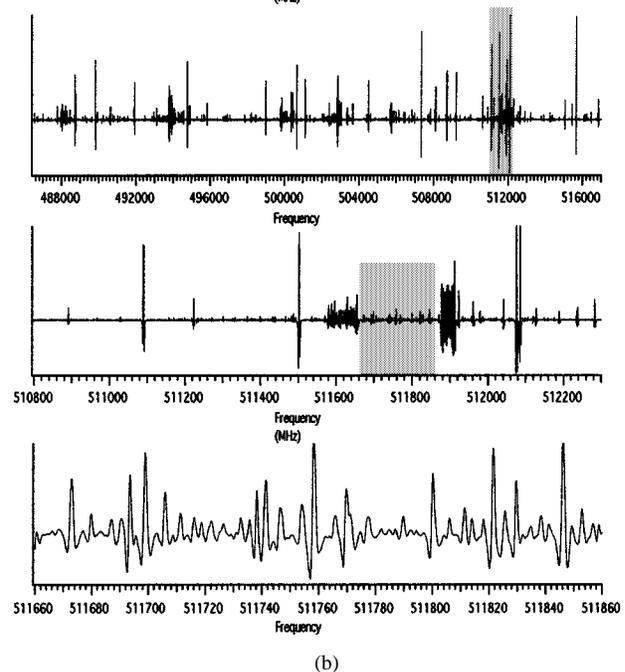
Fig. 7. (a) FASST schematic. (b) Spectral plots at 500 GHz in increasing frequency resolution sweeps (top to bottom) for a combination of pyrrole, pyridine, and sulfur dioxide at 10 mTorr each (courtesy of [43]).
