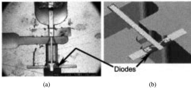
Fig. 18. Terahertz Schottky diode multiplier chips fabricated monolithically from GaAs. (a) 800-GHz balanced doubler with thin membrane frame mounted in waveguide block [171]. (b) 2400-GHz waveguide-mounted substrateless-doubler schematic (currently in process at the JPL) [167].
