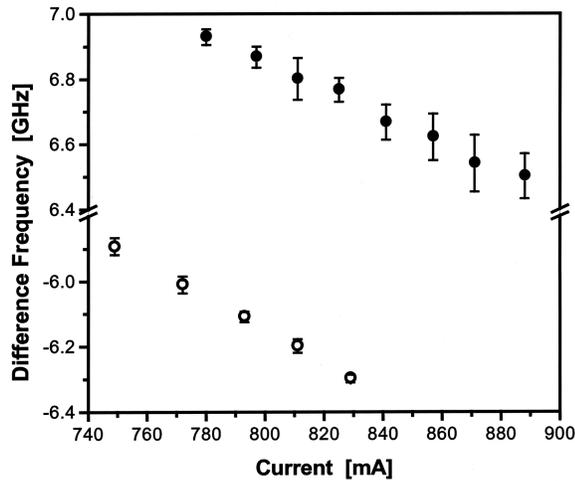
Fig. 4. Tuning of the laser frequency as a function of current for two THz QCLs, both nominally operating at 4.66 THz. The vertical axis shows the difference frequency  $\nu_{\text{QCL}} - \nu_{\text{sum}}$ . Open (filled) circles are for the 100- (200-)  $\mu\text{m}$ -wide laser. The error bars are not due to uncertainty in the measurement but instead indicate the noise broadening illustrated in Fig. 3.
