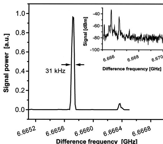
Fig. 2. Typical fast scan of the difference frequency (QCL frequency less 4.6685927 THz). The sweep time for this scan is 3 ms. Inset, the same beat note shown on a log scale. The smaller peaks on either side of the main peak are attributed to instrumentation noise, as in Ref. 13.
