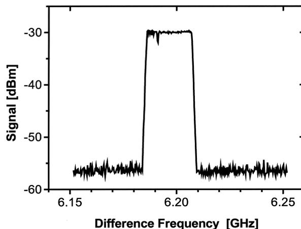
Fig. 3. Measurement of the QCL beat note with the maximum-hold feature of the spectrum analyzer, with a 30-s acquisition time. The 3-dB width of this line is  $\sim 21$  MHz. This illustrates the broadening due to electrical, thermal, and acoustic noise for this unstabilized QCL.
