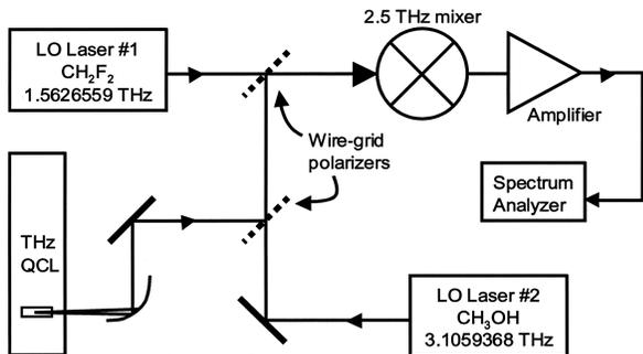
Fig. 1. Diagram of the experimental setup, showing the two independent LOs, whose sum frequency is close to that of the QCL.
