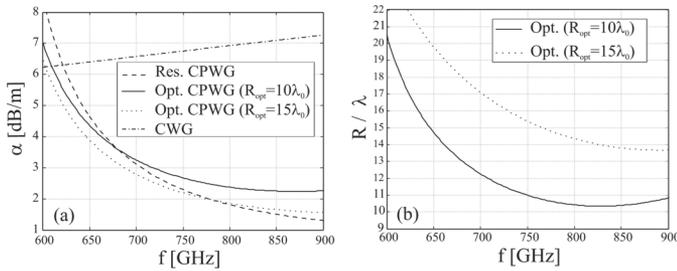
Fig. 3. (a) Propagation loss. The CWG ( $\varnothing = 1.65$  mm.) case considers only conductor losses. (b) Bend radius associated to 1 dB loss for the resulting  $\Delta\beta$ , normalized to the wavelength.
